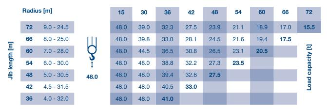
The loads relate to 45 m hook travel. For longer hook travel distances, the loads are reduced by the additional weight of the hoist rope (with 3-rope mode = 12.0 kg/m hook travel).
